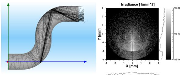
**Figure 2.** Multiple scattering in a metallic pipe modeled with ray-density-weighting. The irradiance distribution behind the pipe is shown on the right side.
