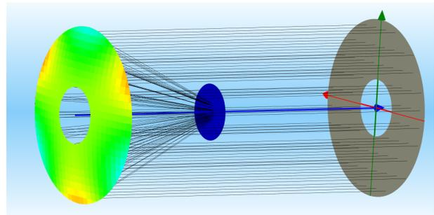
**Figure 3.** Perturbed parabolic mirror, imported from Nastran output files.
